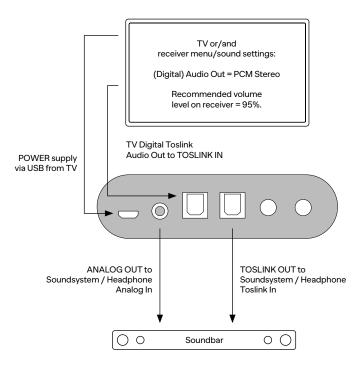
If your TV does not have a "Digital Audio Out/Toslink" with PCM signal, we recommend using an "Analogue to Digital Toslink" converter to connect the analogue output of your TV to our unit.
